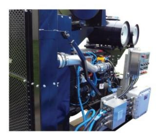
Your equipment regularly needs to operate in hazardous areas and meet international requirements (ATEX, CSA & UL). CMR can develop and customize your products. We routinely develop explosion proof products to operate safely in flammable atmospheres, a particular hazard of methane production and transmission.
